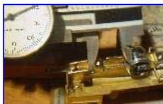
I used my dial calipers to measure the exact distance between the last two drivers. I did this by putting one axle in and then butting the cliper from the front of the axle to the rear of the rear axle slot. That is the exact center to center distance for our side rod holes. The front side rod hole length, I took from the old side rods. These were 1.016 and .710. We'll use these dimensions in a minute but first I made the bottom plate.
