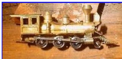
First problem is that the FED 2-6-0 comes with even driver spacing like the D&RGW 2-6-0's. So we need to move the rear axle back under the cab to approximate the California 2-6-0's.
