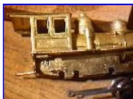
We now have our new axle hole in back. The old axle hole will be covered by a thin piece of brass (or paper) with rivets and brake shoes and a brake cylinder attached. So no need to fill it in. We want to put the fire box details on anyway....so no extra work here.
