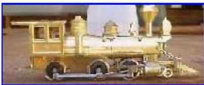
Here are the finished rods installed on the loco. They came out very smooth and because of the accuracy of the rod holes, the mechanism is very smooth. No hitches. I checked the drivers for quarter but they were fine. I had earlier tweaked the frame to get it flat. (when I milled the slot). Let me know if you have any questions....I'll be happy to help if I can.
