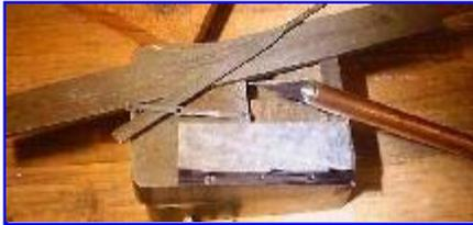
Using a piece of galvanized steel sheet .035 thick (found in the corner of the shop) You can use .030 to .040 brass if you prefer. I like the look of steel. I blackened the surface with a felt pen and then scratched a center line the length of the plate. Then I used the calipers to locate and scratch verticle lines dead on at the side rod hole dimensions. I used a #11 exacto for the scratching.
