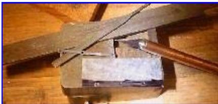
I layed the old rod over the two front holes and scratched around the outside with my exacto. This put the pattern on the metal. I extend those scratches to the new front hole and that put the shape of the rods on the metal. I clamped the metal in a vice and used my jewelers saw to cut out the side rod. I stayed a bit wide and finished to the lines with files. Then I used a big file to clean up the faces (and remove the black)
