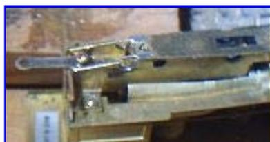
The retainer plate doesn't extend back to cover the new axle position so rather than make a whole new plate, I simply extended the old plate with two pieces of .035 brass wire soldered into two grooves in the plate. I cut the grooves with a dremel and cut off disk. It made perfect grooves for the wire. Once soldered, it was very strong.
